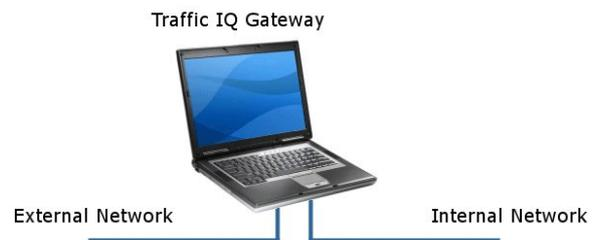
The Traffic IQ Gateway can utilise any virtual or physical adapter and it will bind directly to the chosen adapter thus removing the need to use the operating systems TCP/IP stack. This has numerous advantages and enables the gateway to apply evasion techniques that would not normally be possible.
